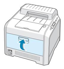
If you have installed the toner cartridges incorrectly, the left cover will not close properly. Check again to make sure the cartridge colors correspond to those marked on the right hand side. Never use force to close the cover.
